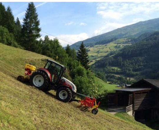
The new GK Series can be used in a split, front-rear mounting.
