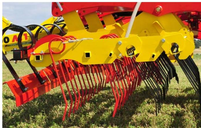
Each of the two rows of heavy gauge tines and two rows of narrower gauge tines lock into position to contribute to pasture maintenance.
