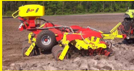
Leveling plates, tines and rollers quickly level soft, tilled soil.
