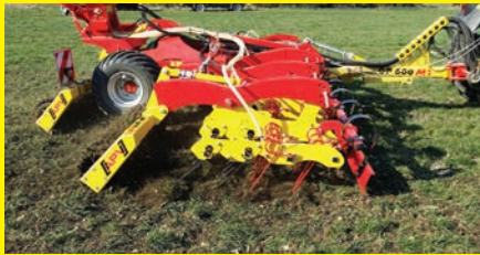
Aggressive tine action provides maximum soil exposure for seeding.
