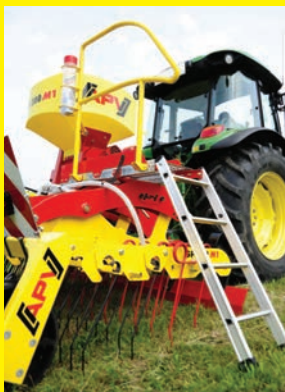
Seeder access platform
