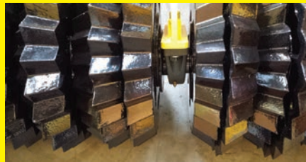
Heavy toothed-ring roller for new till applications and grass management.
