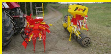
Separation of harrow from roller assembly is accomplished without tools.
