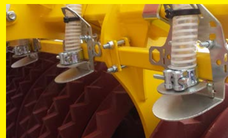
Seed tubes and dispersion plates
