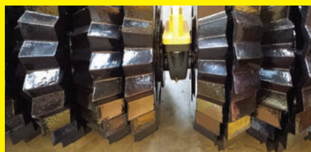
Heavy toothed-ring roller for new till applications and grass management.
