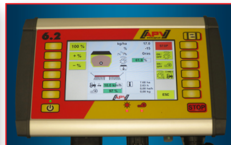
The 6.2 Controller is our most advanced, with touchscreen control.
